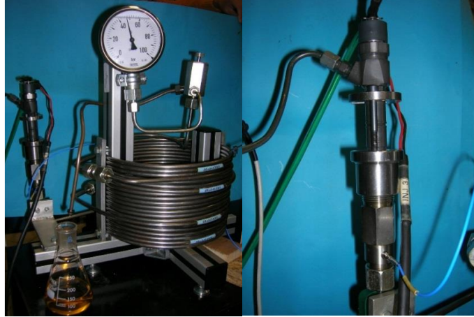
Figure 3.8 - AVL Injection Gauge Rate System.
