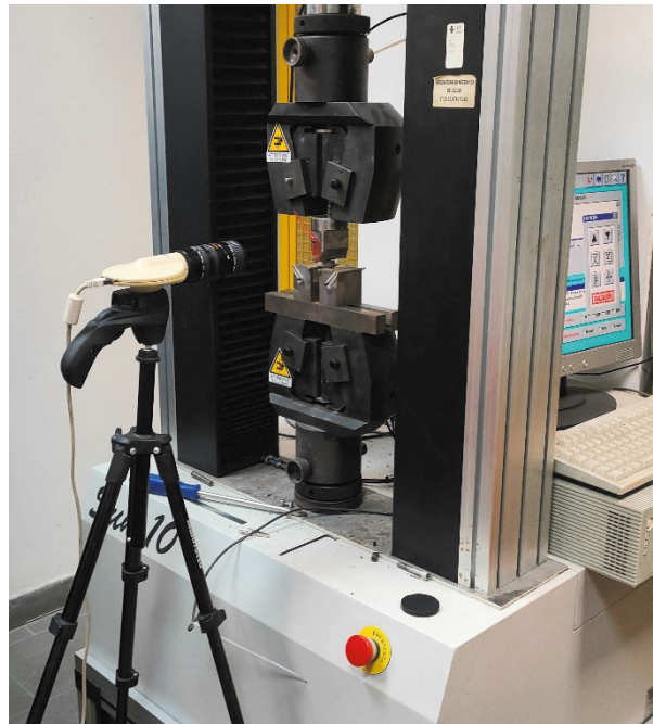
Fig. 2. Experimental equipment for damage monitoring during three-point bending test.
