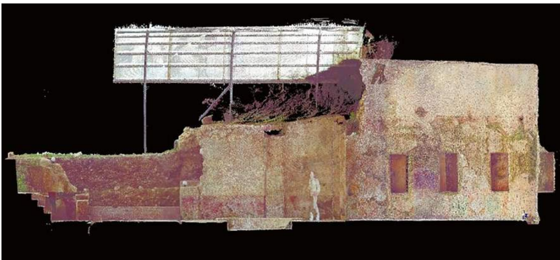
Fig. 9.8 3D processing from point cloud—longitudinal section
