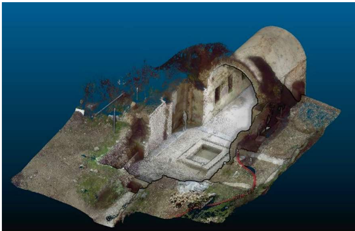
Fig. 9.1 3D point cloud processing with textures
