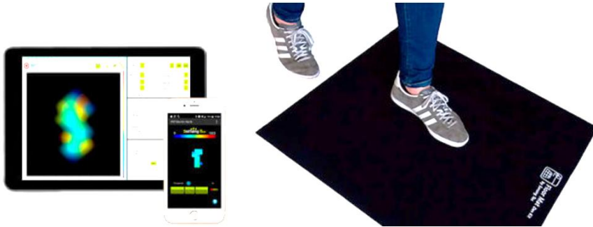
Figure 5.16 Example of a pressure-sensitive floor system used for footstep detection and pressure mapping
