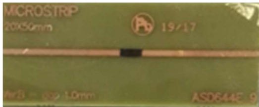
Fig. 3. A picture of the realized microstrip embedding a film of carbon nanotubes (black patch).
