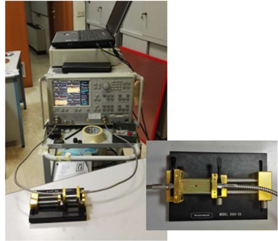
Fig. 6. The set-up for the microwave characterization: the Vector Network Analyzer is connected to the test fixture (magnified in the inset).
