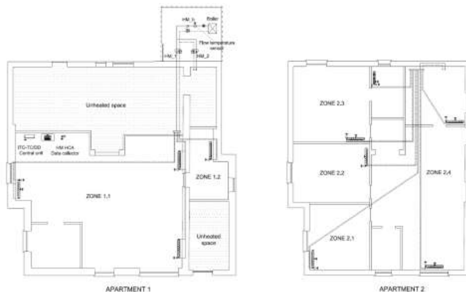
Figure 1.6 – Heating plant scheme of the two-family house
