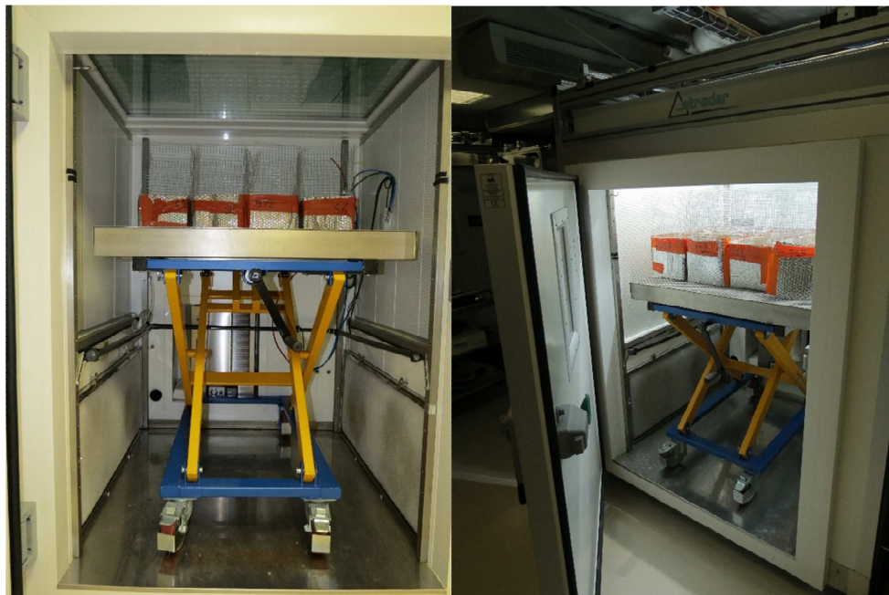
517 518 Figure S3 : Pots positioned in the growing chamber at a fix distance from lights in the Ecotron facilities
