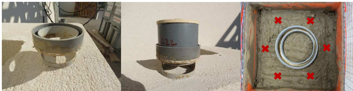
514 515 Figure S2 : From left to right: example of the ring used for soil respiration analysis, ring with the plastic dome in place 516 and ring inside the soil, the red crosses mark the spots were the seeds were planted
