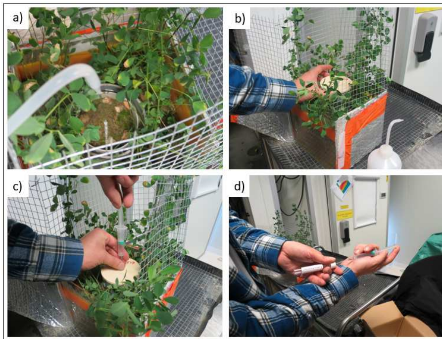
528 Figure S7 : Air sampling protocol : a) fill ring with water, b) place the plastic cap on top, c) take a 5ml air samples using 529 a syringe on the rubber cap and d) transfer the air taken in the airtight exainers
