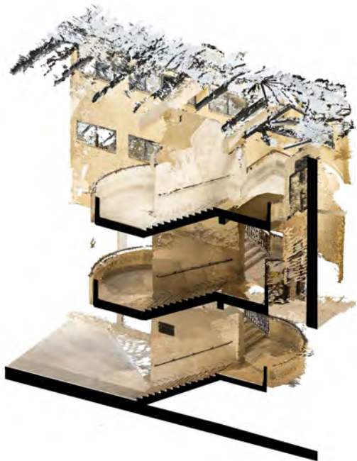
Figure 7: Detail of the point cloud of the stairs.
