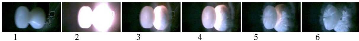
Figure 1. Sequence of light emission in impact of nylon sabot at 200 m/s with 40 mm gun bore.
