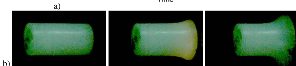
Figure 4. a) Measured light emission intensity vs time for nylon on steel anvil impact at 260 m/s and b) sequence of high speed camera recording showing light emission at contact.
