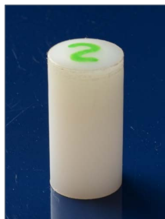
Figure 2. Example of nylon Taylor cylinder used to measure light emission under impact
