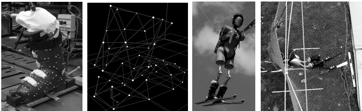
Figure 1. (a,b) Experimental deflection analysis on boots by means of motion capture systems. (c,d) Experimental analysis of instrumented anthropomorphic dummies against nets and safety barriers.
