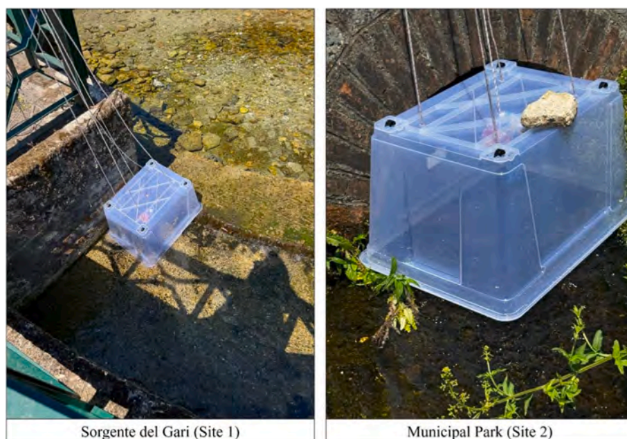
Fig. 3. Experimental apparatus deployed to evaluate the radon emission rate of the unit area of the two springs (Sites 1 and 2).
