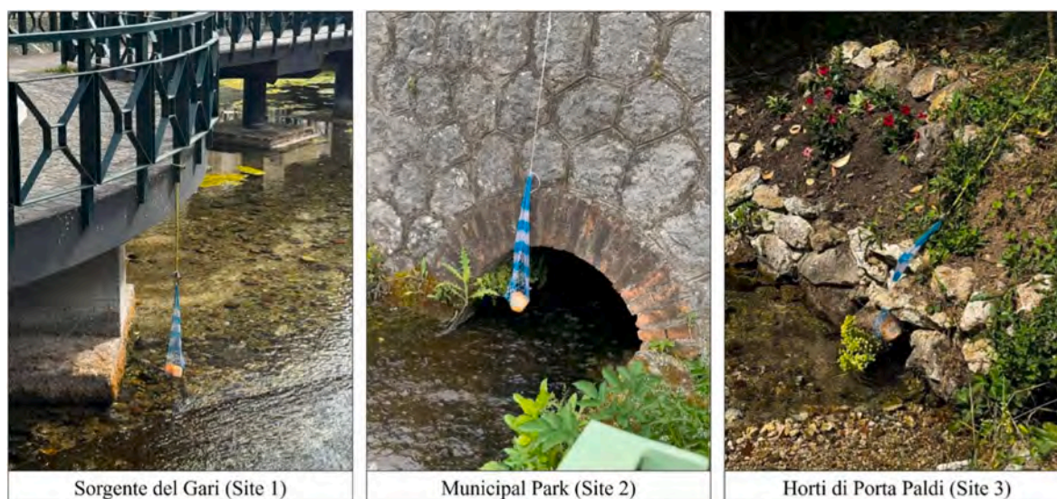
Fig. 2. Details of the positioning of the sensor for in situ measurements at the three different springs.
