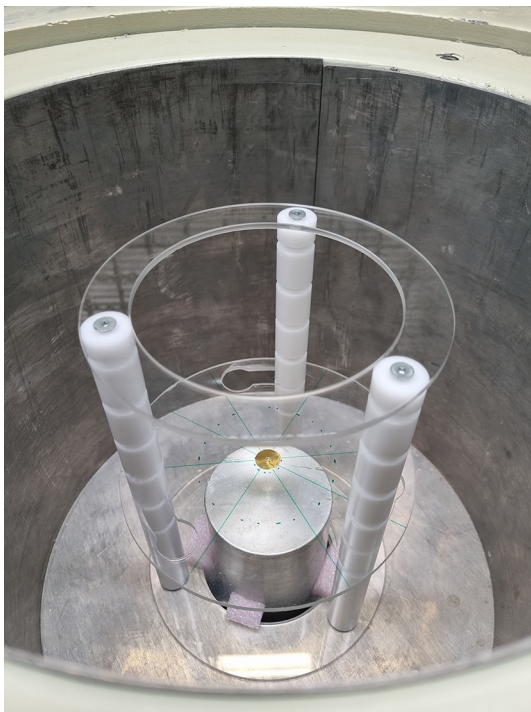
Fig. 9 Gamma spectroscopy station with the HPGe detector and the surrounding lead shielding. A thin methacrylate support was used to position the samples. A gold foil is shown in the sample position at 3 cm from the detector
