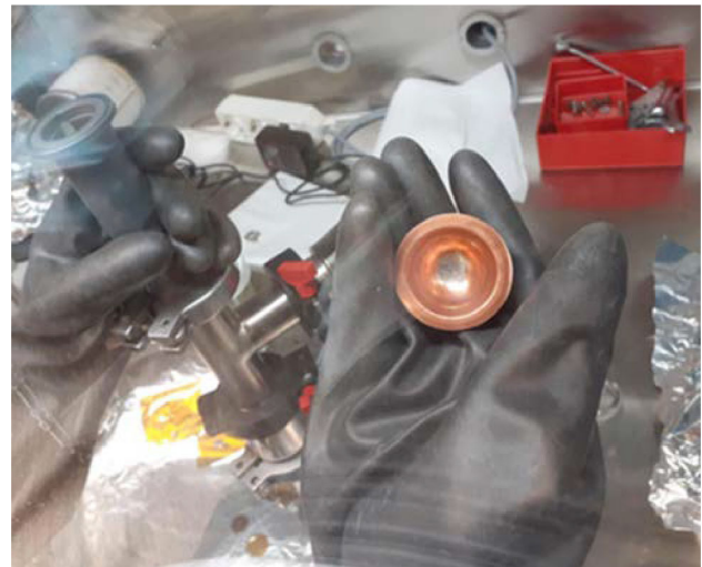
Fig. 3 Lithium pressed into a 300 \mu\text{m} thick copper backing and beam stopper. The production procedure, carried out inside an argon glovebox, is described in Sect. 2.4
