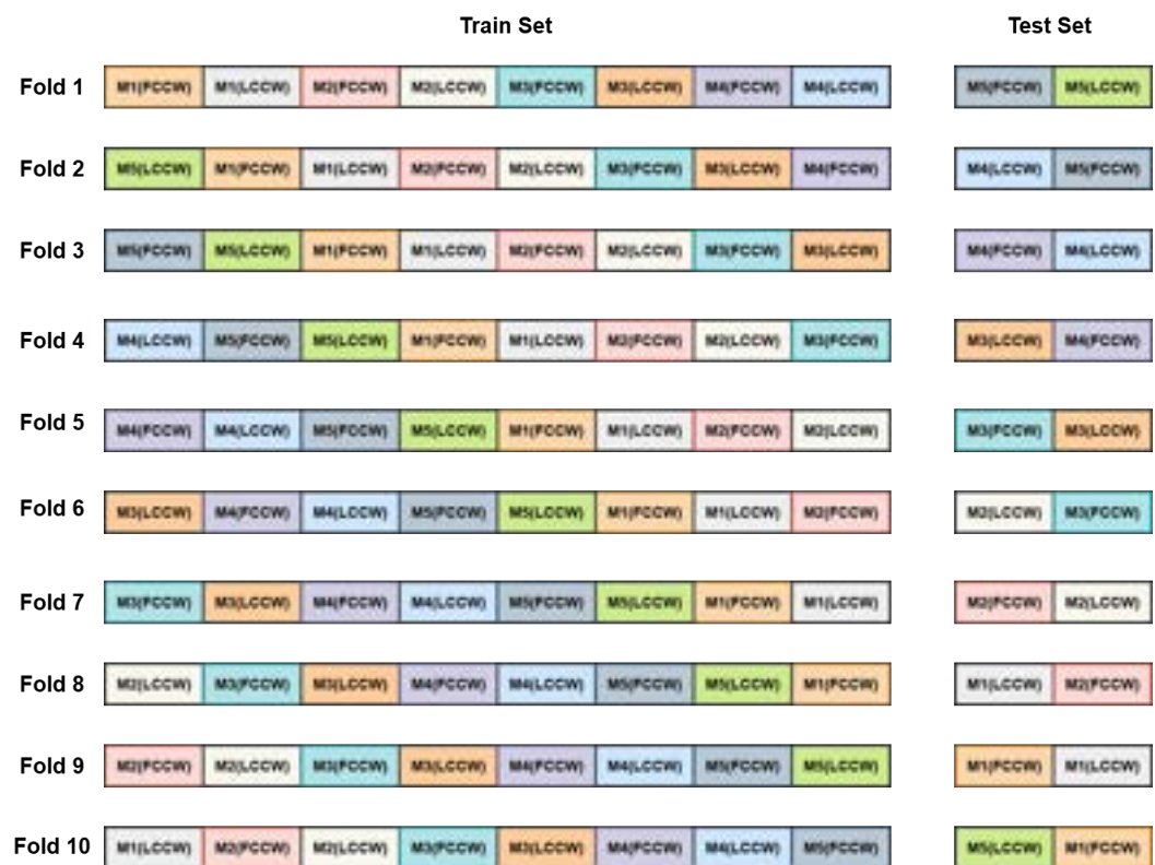
Figure 14. Stratified 10-fold cross-validation across 102 classes adopted for combined data. Each row represents the fold, and each column represents the measurement. In each fold, two measurements per class are used for testing from FCCW and LCCW, and the remaining eight are used for training.
