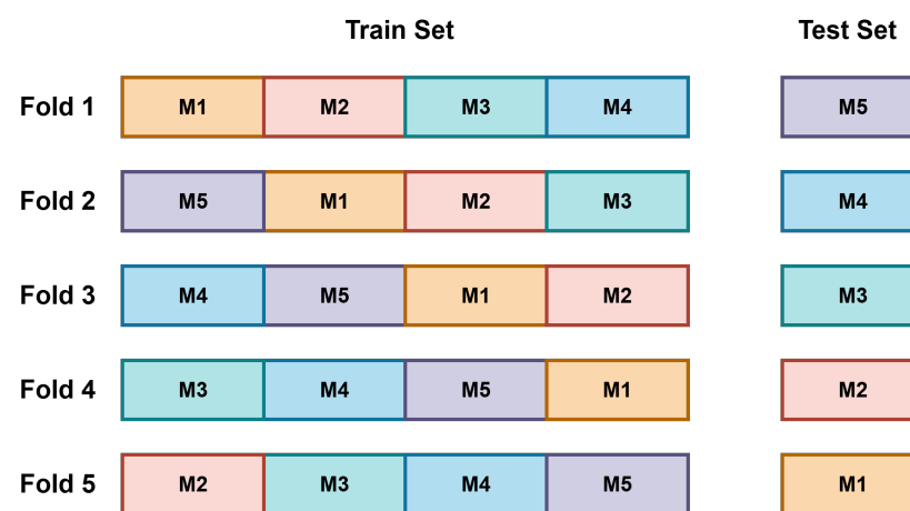
Figure 13. Stratified 5-fold cross-validation across 102 classes adopted for LCCW and FCCW data. Each row represents the fold, and each column represents the measurement. In each fold, one measurement per class is used for testing, and the remaining four are used for training.
