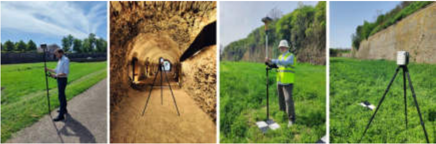
Fig. 2 – Survey phases: from the left GNSS and TLS acquisition in Lucca and GNSS and TLS acquisition in Alessandria. (Source: created by the authors)
