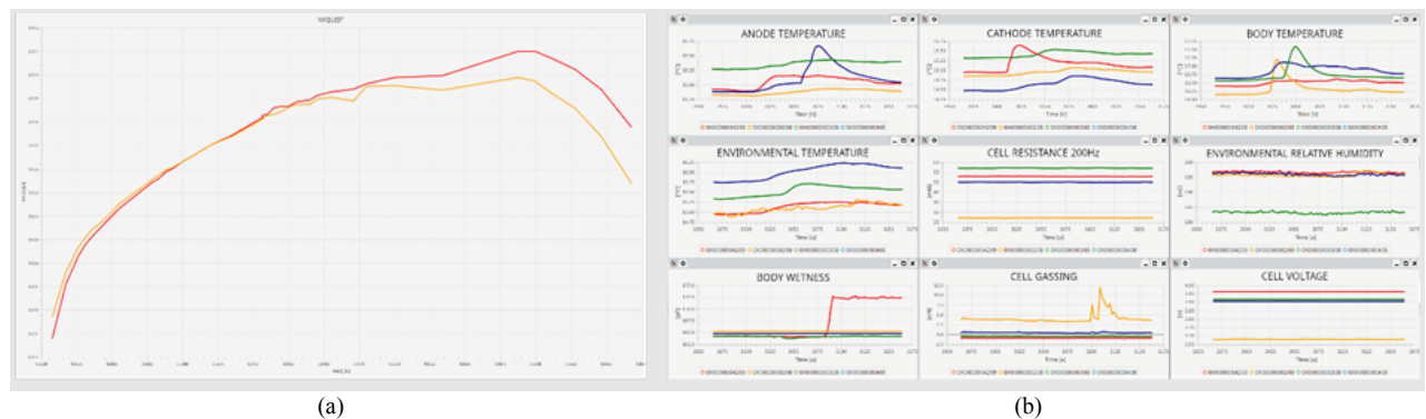
Figure 7. (a) internal cell impedance Nyquist graph in the range 5Hz – 20kHz performed on two cells simultaneously; (b) screenshot of nine different measurements (four temperatures, internal cell impedance at 200Hz, relative humidity, body wetness, cell gassing and cell voltage) performed on four cells simultaneously.
