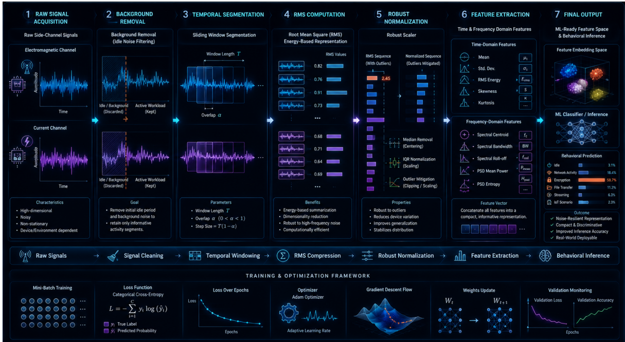
Figure C.1: Overview of the RMS-based preprocessing pipeline adopted for side-channel behavioral inference. Raw electromagnetic and current-consumption signals are processed through background removal, temporal segmentation, RMS computation, robust normalization, and feature extraction stages in order to generate compact and noise-resilient feature representations suitable for machine learning classification.
