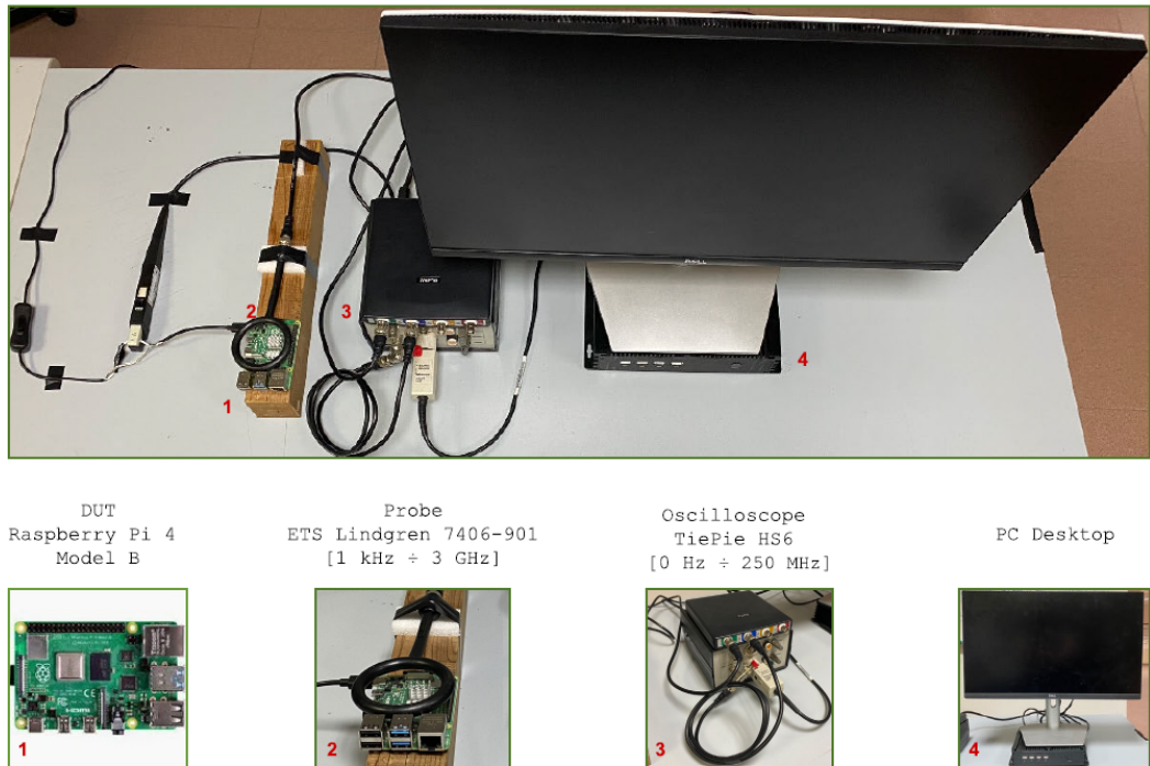
Figure 3.1: Experimental setup for electromagnetic side-channel measurement. (1) Device Under Test (Raspberry Pi 4 Model B); (2) Magnetic Field Probe (ETS Lindgren 7406-901); (3) Oscilloscope (TiePie HS6); (4) Acquisition and control PC.
