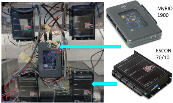
FIGURE 5 | Controller unit consisting of MyRIO 1900 and four servoamplifiers ESCON 70/10.
