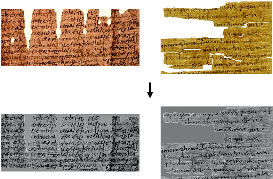
Fig. 1: Processing on original images turned into greyscale with background uniformity.
