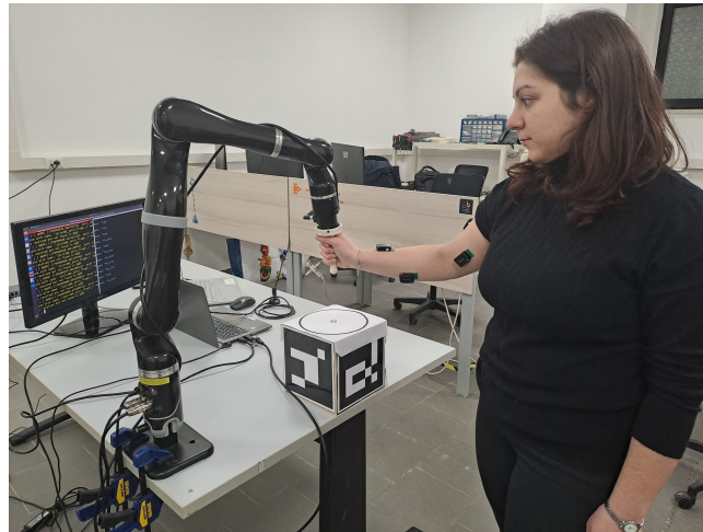
Figure 3. The scenario shows the experimental setup in which a human operator performs a co-manipulation task using a Jaco 2 manipulator. On the dominant arm of the human operator, four Delsys Trigno Avanti EMG sensors are placed on the biceps and triceps brachii, flexor carpi radialis and extensor carpi ulnaris muscles.
