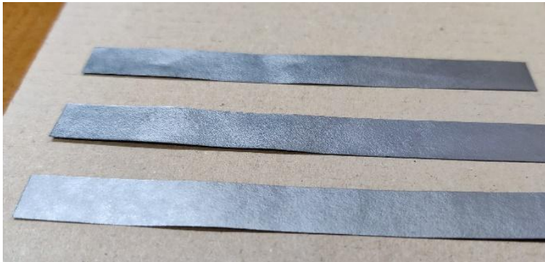
Figure 10. Nanocomposite strips derived from macroscopic graphene nanoplatelet sheets (Giovinco, 2023).
