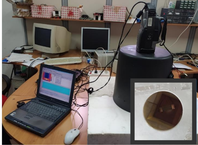
Figure 19. Schematic (a) and picture (b) of the set-up for the estimation of the emissivity of the material under test (Sibilia, 2021).
