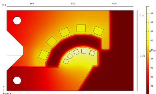
Fig. 5. Simulated temperature distribution for case II @ T_{AMB,MAX} = 80\text{ }^{\circ}\text{C} , t = 20\text{ s} . (For interpretation of the references to colour in this figure legend, the reader is referred to the web version of this article.)
