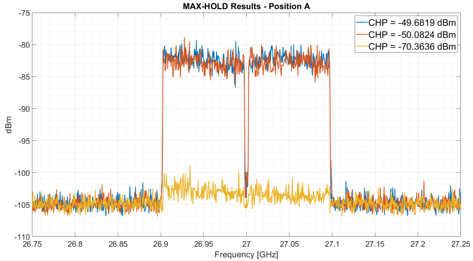
Figure 3.25 – Max-hold results obtained at position A for each activation stage in the FR2 measurement campaign: only CPE 2 activated (blue line), both CPEs active (red line), only CPE 1 active (orange line).
