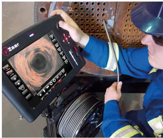
Figure 2.2: Non-destructive inspection using the visual inspection technique.
