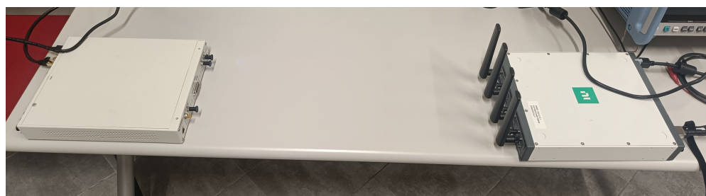
Figure 3. Ettus Research USRP X310, and NI Ettus USRP X410 on the right.
