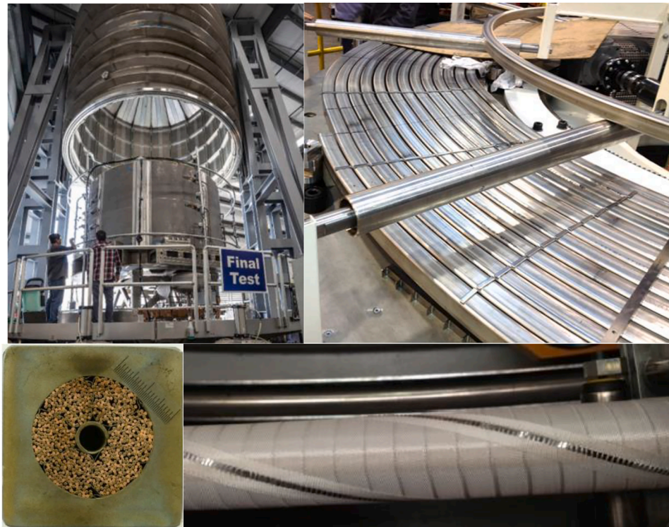
Fig. 1. Top left – CS module 1 during assembly into the test facility at GA/USA, top right: CS module dummy winding trial, bottom left: cross-section of the CS conductor, bottom right: CWT assembly over the conductor insulation.
