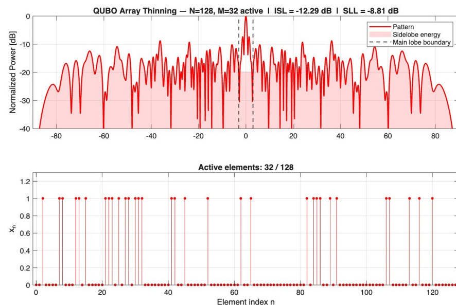
Figure 2. Normalized radiation pattern of the QUBO-thinned array ( N = 128 , M = 32 , d = \lambda/2 ). The shaded region indicates the sidelobe area used in the ISL computation ( 10^\circ < |\theta| \leq 90^\circ ).
