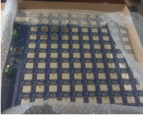
FIGURE 1.2: Photograph of a practical reconfigurable intelligent surface prototype.
