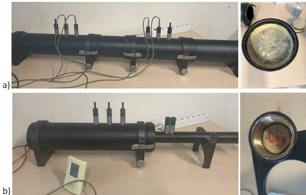
Figure 6. Configuration of a) large tube for transmission loss b) small tube for absorption
