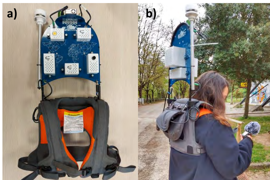
Figure 1. Wearable system used for monitoring the environments: front view (a), and system in use (b).
