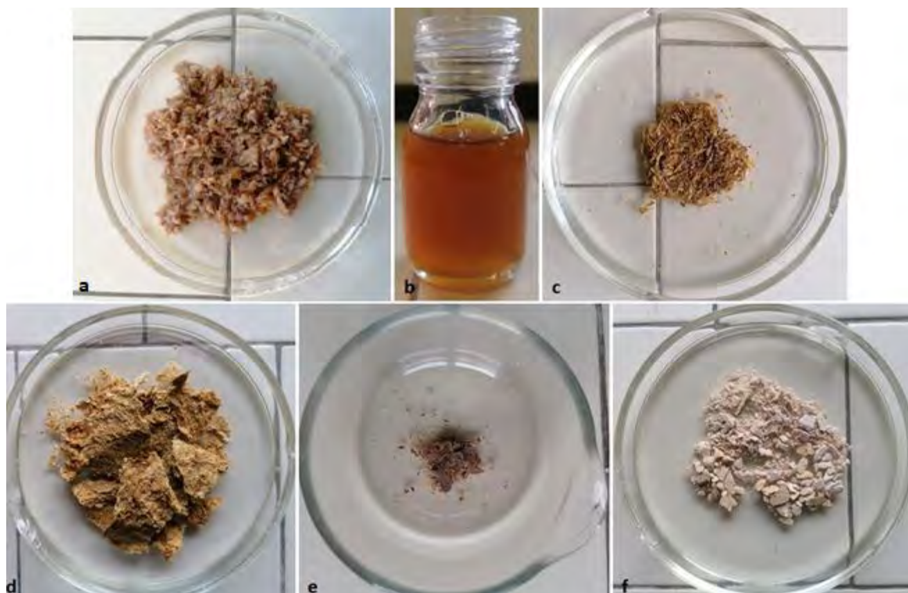
Figure 2. BSG as it is (a), protein fraction (b), fibrous fraction (c), cellulose (d), lignin (e) and functionalized arabinoxylan (f).
