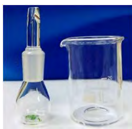
Figure 1. Pycnometer used for the density measurements.
