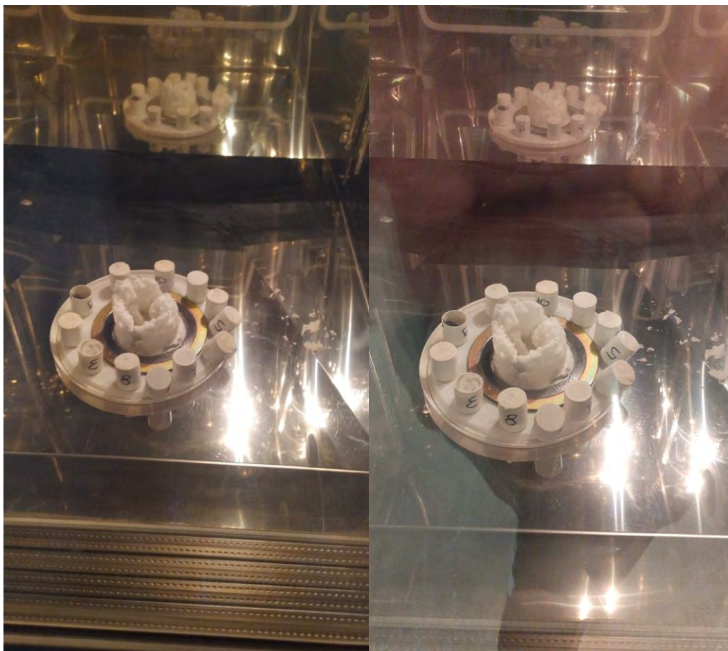
Figure 3. Hydrate samples in 3D printed casing.
