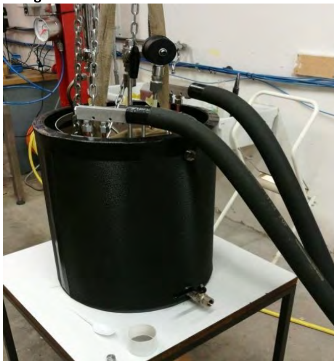
Figure 2. Reactor in the thermostatic bath.
