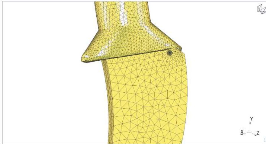
Figure 17: Case 2A mesh (crack depth: 2.6mm).
