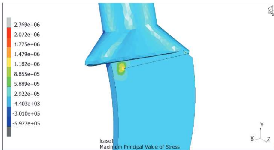
Figure 22: Case 2C Maximum principal value of stress distribution at t=0.19s .
