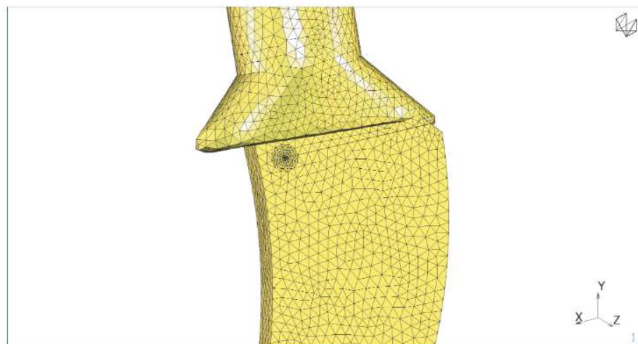
Figure 19: Case 2C mesh (crack depth: 14.3mm).
