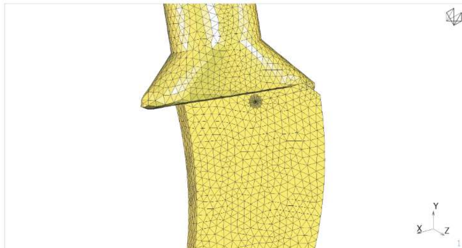
Figure 18: Case 2B mesh (crack depth: 8mm).
