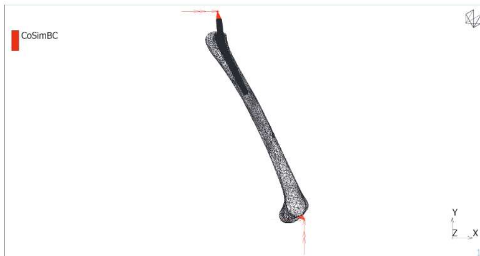
Figure 4: Boundary conditions for the FEM model.
