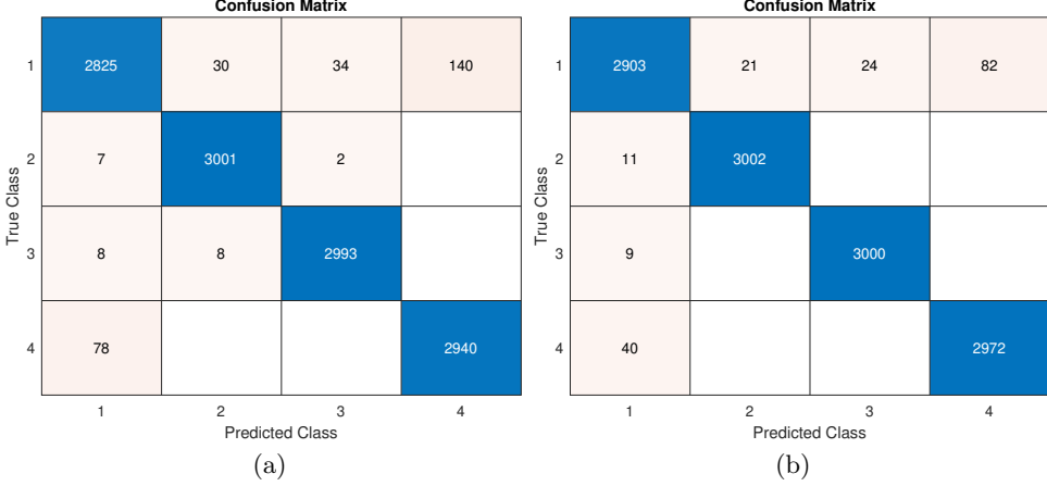
Figure 3.9: Confusion Matrix of test phase: (a) Considering acceleration data from all axis; (b) Considering acceleration and angular velocity data from all axis
