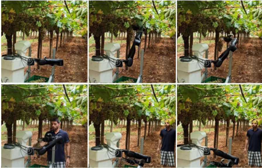
Figure 4.7: Snapshots of human-robot safety experiments in realistic conditions with robot performing a single-arm harvesting operation. Top figures shows the robot performing the grape harvesting without the human intervention. Bottom figures show the human approaching the harvested grape (and the robot) to taste it.
