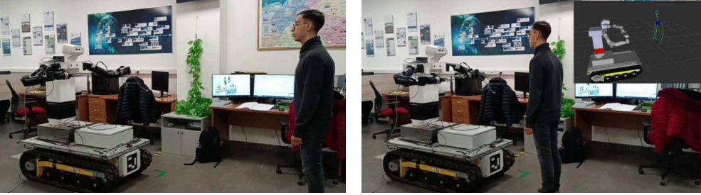
Figure 4.3: Two snapshots of the robot performing a cooperative motion in laboratory environment. On the left, the operator is far enough from the robot such as the safety field is above the considered threshold. On the right, the operator gets close to the robot making the robot modify the nominal trajectory.
