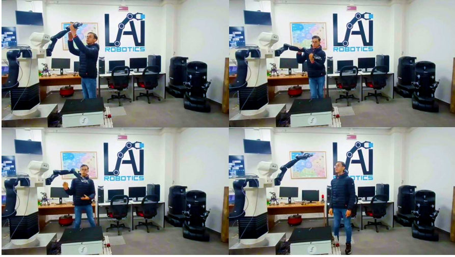
Figure 4.11: Screenshot of the video showing the admittance control experiment. Top Left: the human operator starts physically interacting with the end-effector. Top Right: the human operator pulls down the end-effector. Bottom Left: the human operator stops interacting with the end-effector. Bottom Right: the end-effector returns to the desired position.
