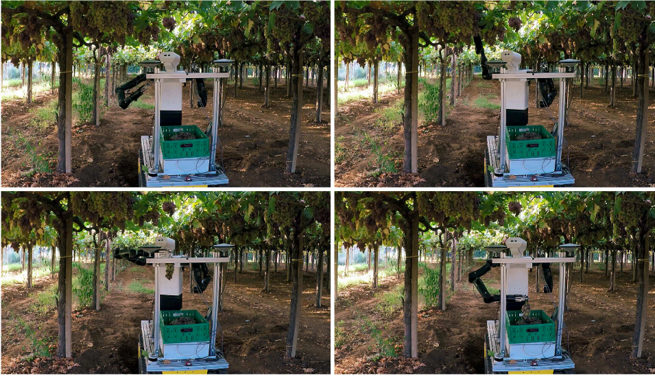
Figure 4.19: Top Left: image of the robot with both harvesting tools in the home configuration. Top Right: image of the robot with the right harvesting tool in the pre-grasp position. Bottom left: image of the robot with the right harvesting tool in the pre-release position. Bottom right: image of the robot with the right harvesting tool in the release position.
