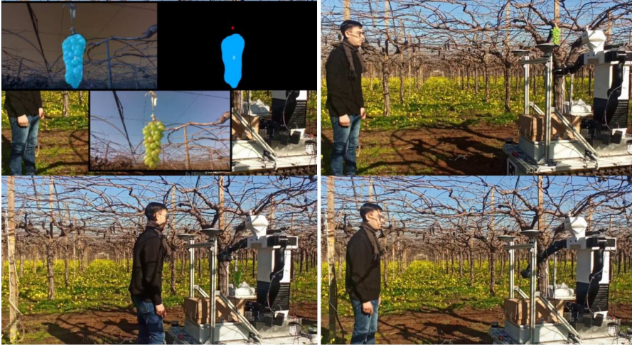
Figure 4.6: Snapshots of human-robot safety experiments in representative conditions with robot performing a single-arm harvesting operation. Top Left: results of the grape perception for the planning of the nominal agronomic trajectories. Top Right: the robot starts the agronomic harvesting while the operator is far away from the robot. Bottom Left: the operator get close to the robot while it grasps the harvested grape. Bottom Right: the operator moves away from the robot that releases the grape in the box.
