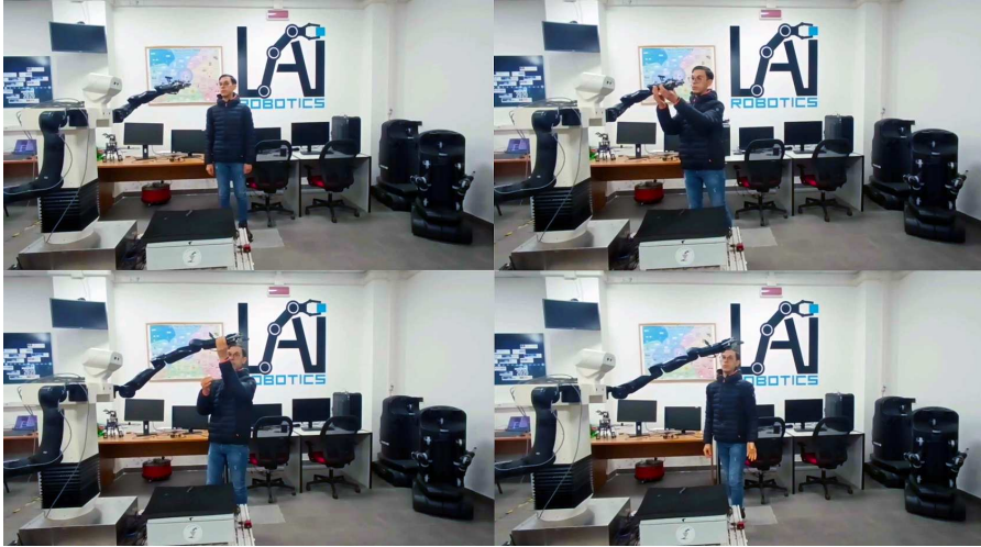
Figure 4.15: Screenshot of the video showing the hand-guiding control experiment. Top Left: the human operator gets close to the robot. Top Right: the human operator starts physically interacting with the end-effector. Bottom Left: the human operator pulls up the end-effector. Bottom Right: the human operator stops interacting with the end-effector and it remains still.
