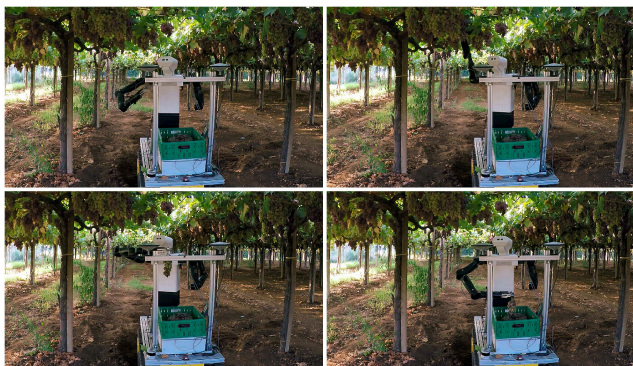
Figure 3.16: Top-left) Image of the robot with both harvesting tools in the home configuration. Top-right: image of the robot with the right harvesting tool in the pre-grasp position. Bottom-left) Image of the robot with the right harvesting tool in the pre-release position. Bottom-right) Image of the robot with the right harvesting tool in the release position.
