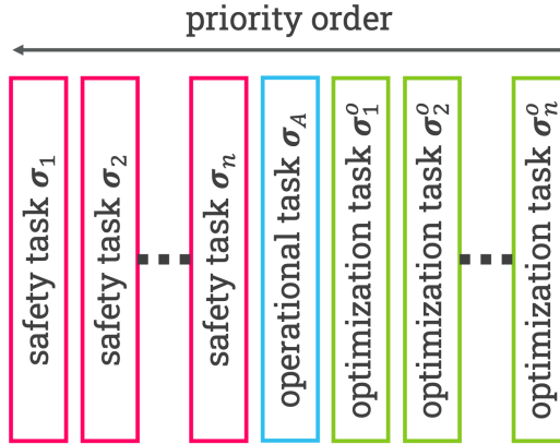
Figure 2.1: Example of hierarchy with tasks grouped into three categories. Priority decreases from left to right, with safety tasks having higher priority than operational and optimization tasks.
