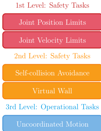
Figure 3.9: The task hierarchy used to validate the uncooperative motion operational task described in Section 3.4.4.
