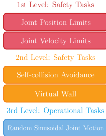
Figure 3.5: The task hierarchy employed to validate the safety tasks introduced in Sections 3.4.1-3.4.3.
