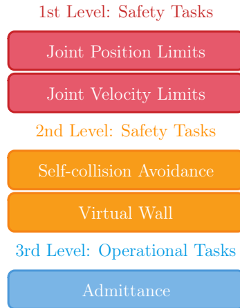
Figure 4.10: The task hierarchy used to validate the operational task described in Section 4.3.2.1.
