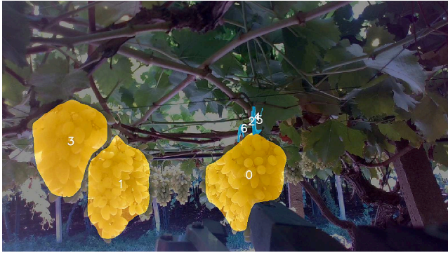
Figure 3.15: Output of the perception system. The highlighted zones represent the grapes (yellow zones) and the peduncles (light-blue zones) that the software has detected, with a confidence score above 0.9.
