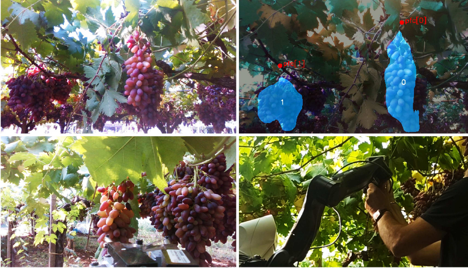
Figure 4.21: Top Left: image of the grapes from the robot’s head camera. Top Right: result of the grape recognition and peduncle localization process. Bottom left: images of grapes taken from the right wrist camera. Bottom Right: human operator assisting the robot during the harvesting procedure.
