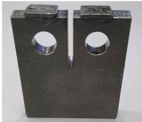
Fig. 1. CT specimen for fatigue crack propagation test.
