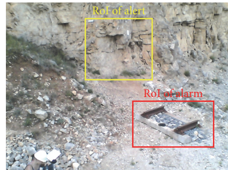
FIGURE 8: Point of view of AiCP. The RoI of alert is in the yellow frame and the Roi of alarm in the red one.
