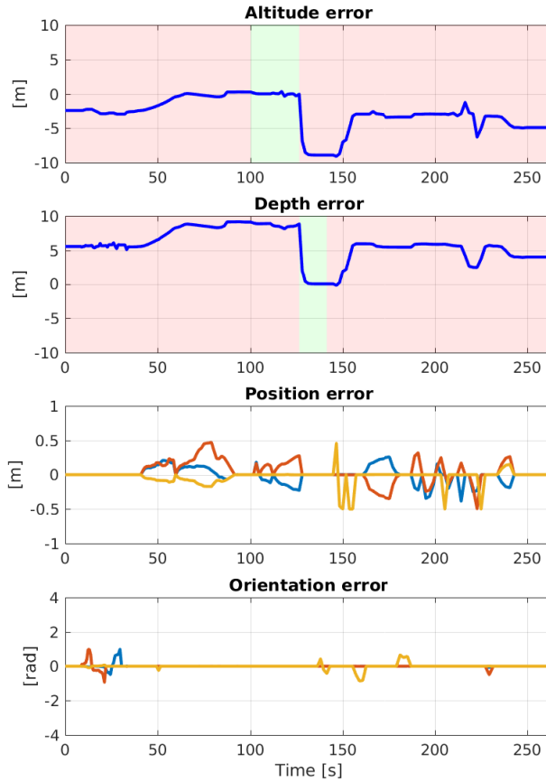
Figure 4.20: Task error plots: altitude ( m = 1 ), depth ( m = 1 ), position ( m = 3 ) and orientation ( m = 3 ). The green and pink background represents the enabled and disabled state, respectively, of the corresponding task.
